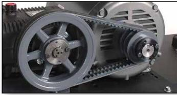
■ **Belt Pulley System** with notched V-belts and cast iron pulleys reduce belt slippage and offer longer belt life with cooler operation.
